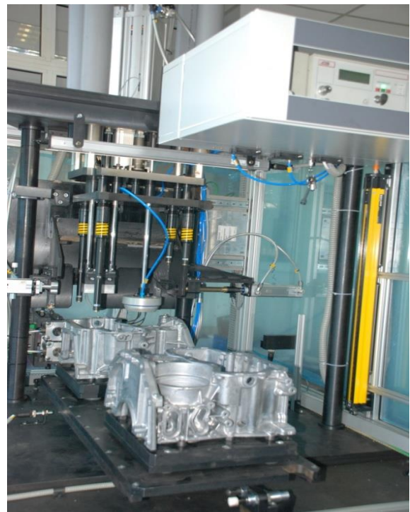
Pre-machined smart mechatronic leakproofness control system Semel H5-GEN.2
